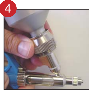
Tighten swivel cap and secure bottle
