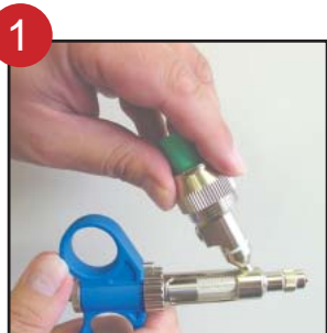
Unscrew the bottle nut two turns only
