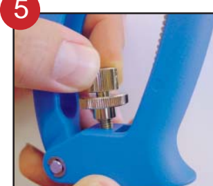
Turn dosing adjustment screw to set the required dosage. Retighten lock nut
