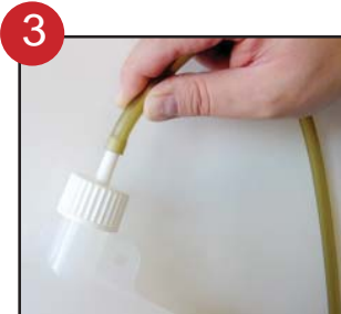
Option 2: Attach the other end of the amber tube to the 2.5 liter backpack
